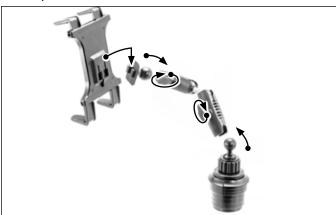
3 Twist ribbed collar counterclockwise to expand base to fit cup holder as needed.
