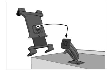
3 Insert tablet by placing it on the two lower legs and pushing down on the spring-loaded bottom of the holder. Loosen adjustment knob to adjust rotation, position, or angle. Retighten to set.
