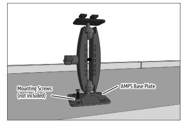
Insert tablet by placing it on the two lower legs and pushing down on the spring-loaded bottom of the holder. Loosen adjustment knob to adjust rotation, position, or angle. Retighten to set.
