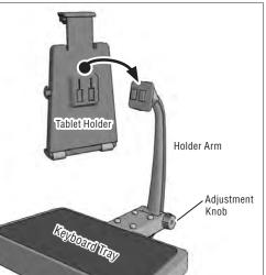
Insert tablet into holder and place keyboard on the tray.
