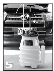
Turn the handle on top of the (-02) upper cover. (Check before the operation. 4. Check if the tube is inserted to the bottom of the engine.)
