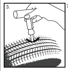
3. Insert the tire repair string (tire plug) into the hole and push straight down on the insert tool handle till the ends of the tire repair string (tire plug) are sticking out of the tire 1/2" to 1" (13-25mm).
