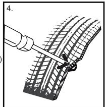
4. Pull the Heavy-Duty Steel T-handle Insert Tool straight out of the hole till the tip is just even with the tire tread then cut the exposed tire plug ends just slightly above the tread and remove the installation tool.
