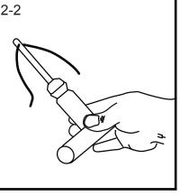
2. Prepare Heavy-Duty Steel T-handle Insert Tool for insertion by first dipping the tip into the lubricant. 2-1. Next insert the tire repair string (tire plug) through the hole in the installer tool.
