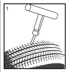
1. Insert the Heavy-Duty Steel T-handle Spiral Probe Reamer into the punctured tread at a slight angle then straighten the reamer and push the tapered shaft in and out of the hole several times to expand and enlarge the broken steel cord.
