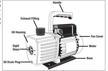
This vacuum pump has been tested at the factory and shipped with only trace amounts of oil. **OIL MUST BE ADDED BEFORE OPERATING!** Failure to add oil will damage cartridge and void warranty!
