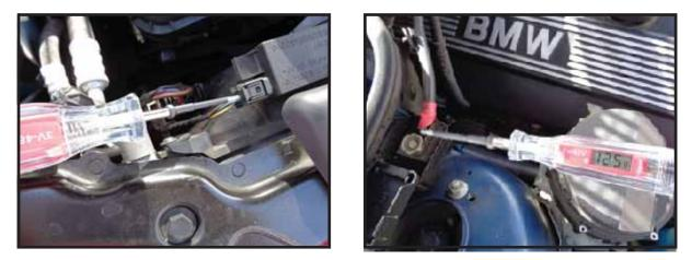
For smaller circuits where exacting precision is required, you can use a precision screwdriver or similar tool as a ground probe, connecting the ground to the end of the probe, while using the probe as the positive lead.
