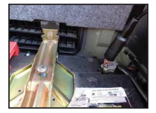
Using the probe end or clips, you are now ready to test your circuit. Touch your probe tip to the electrical point that is in question to get your voltage reading.
