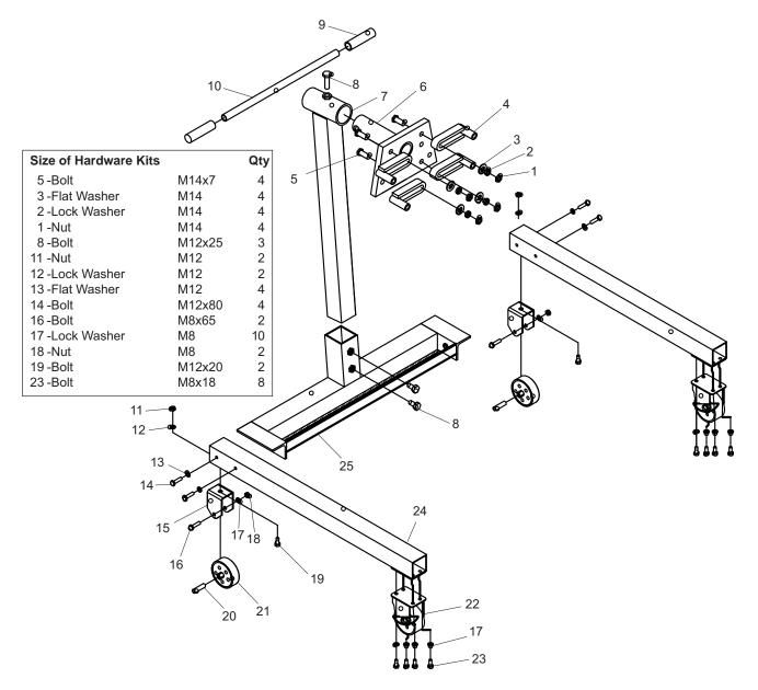
Figure 2 - Assembly Illustration for Model ATD-7482
