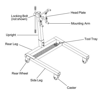
Figure 1 - Model ATD-7482 Engine Stand components
