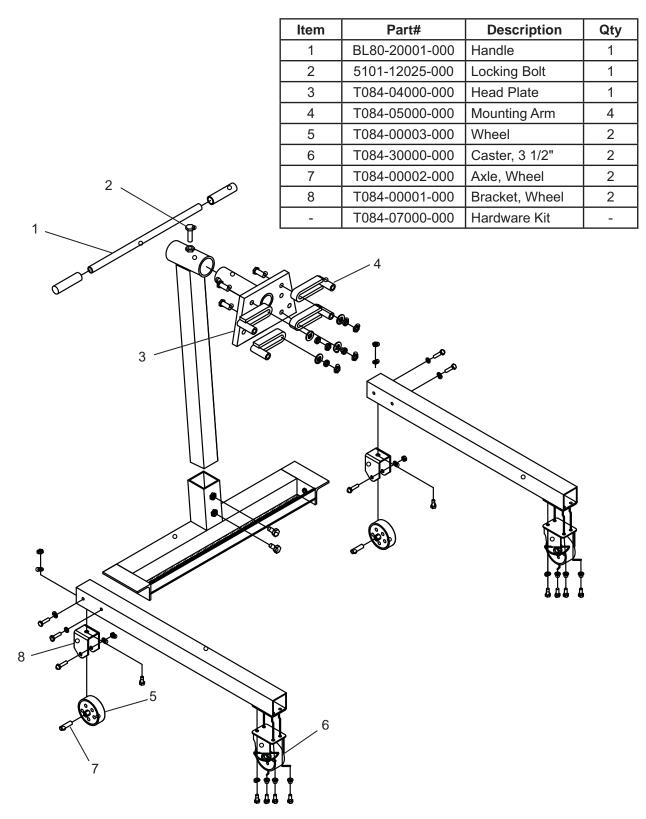
Figure 3 - Replacement Parts Illustration for model ATD-7482
