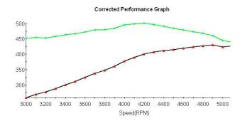
**Cam Specs:** 220/224 @50 .512in/.512ex 112LSA **Cylinder Heads:** Edelbrock Aluminum 60cc 2.02/1.60
