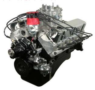
HP: 430 @ 5400RPM TQ: 500 @ 4000RPM Block: OE Ford Roller Block Bore/Stroke: 4.040 x 4.000 Crankshaft: Scat Nodular Steel Rods: Scat 4340 I Beam
