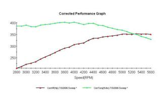
**HP:** 350 @ 5200RPM **TQ:** 400 @ 4000RPM
