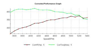
**HP:** 375 @ 5200RPM **TQ:** 415 @ 4100RPM
