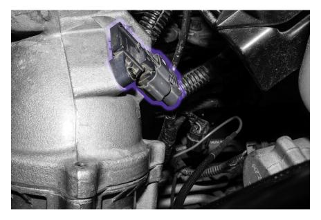
3. Unplug the factory connection and plug the Boost Fooler in line as shown in figure 3.
