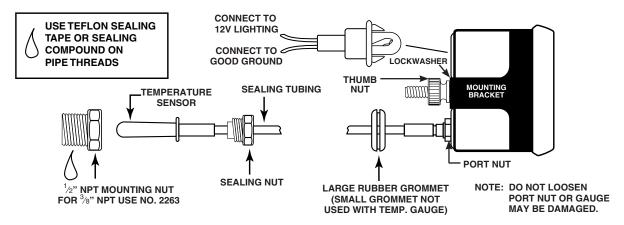
**NOTE:** Some late model vehicles use electronic sensors in their pressure and temperature senders for engine control functions. Before removing the original sender, we recommend that you contact your automotive dealer to be sure no critical functions will be disrupted.
