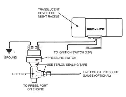
\* Some pressure & temperature switches are internally grounded (one terminal) and do not need a separate ground wire. It is necessary for these switches to be mounted in a good grounded location in order for the Pro-Lite to function correctly.
