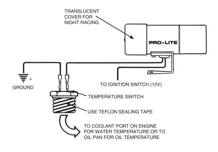
**IMPORTANT:** Some late model vehicles use electric sensors in their pressure and temperature switches for engine control functions. Before removing the original switch, we recommend that you contact your automotive dealer to be sure no critical functions will be disrupted.
