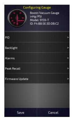
PID – Use to select the PID you would like the gauge to report
