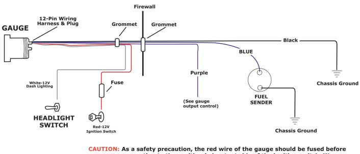
connecting to the positive (+) output side of the ignition switch. We recommend using a 3 Amp, automotive type fuse inline between the power supply source and the red wire of the gauge.
