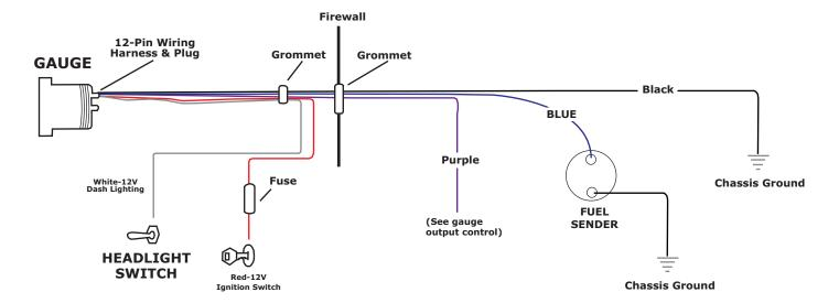
CAUTION: As a safety precaution, the red wire of the gauge should be fused before connecting to the positive (+) output side of the ignition switch. We recommend using a 3 Amp, automotive type fuse inline between the power supply source and the red wire of the gauge.
