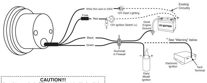
As a safety precaution the RED wire of this product should be fused before connecting it to the positive (+) side of the 12V DC battery. We recommend using a 1 Amp, 3AG fast-acting type cartridge fuse (Littlefuse® #312 001 or an equivalent) inline with the RED wire of our product.
