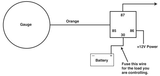
Power for load, EX electric motor, Solenoid, Incandescent Light, LED Light, etc. For wires going to terminals 30 & 87, use proper sized wire for the load you are operating. Terminal 86 can use 18G or 20G wire.
