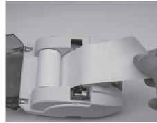
3. Close lid by pushing on both sides of the printer cover at the lid tabs until you hear a snap. Paper is loaded and ready to use.
