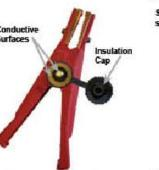
WARNING insulation cap must be installed (on red clamp) when performing in vehicle test to prevent potential arcing.
