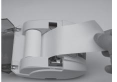
3. Close lid by pushing on both sides of the printer cover at the lid tabs until you hear a snap. Paper is loaded and ready to use.
