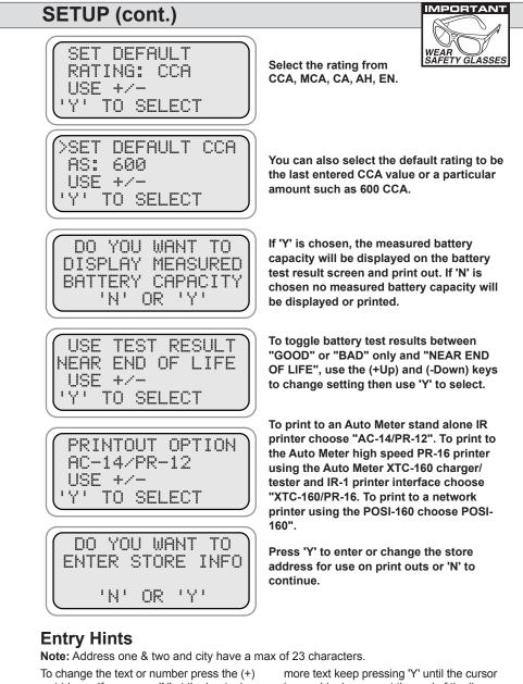
To change the text or number press the (+) or (-) keys. If you press 'N' at the beginning of the screen, no changes will be made. To make changes, use the (+) and (-) keys then press 'Y' to save the change. The cursor will then go to the next character or number. If you are done making changes but there is
