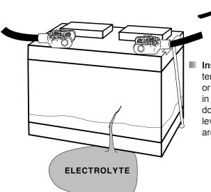
Inspect Battery for terminal corrosion, loose or broken posts, cracks in the case, loose holddowns, low electrolyte level, moisture and dirt around the terminals.
