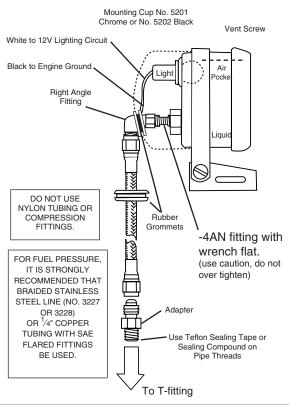
position. Remove dust plug and quickly thread braided tubing into isolator port (be careful not to spill any fluid).
