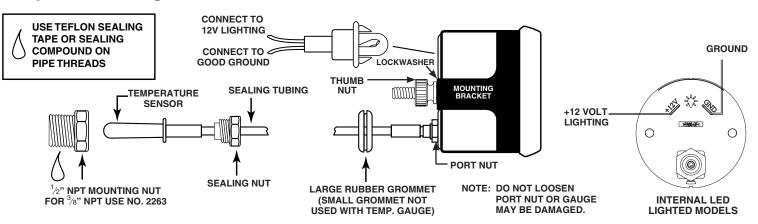
**NOTE:** Some late model vehicles use electronic sensors in their pressure and temperature senders for engine control functions. Before removing the original sender, we recommend that you contact your automotive dealer to be sure no critical functions will be disrupted.
