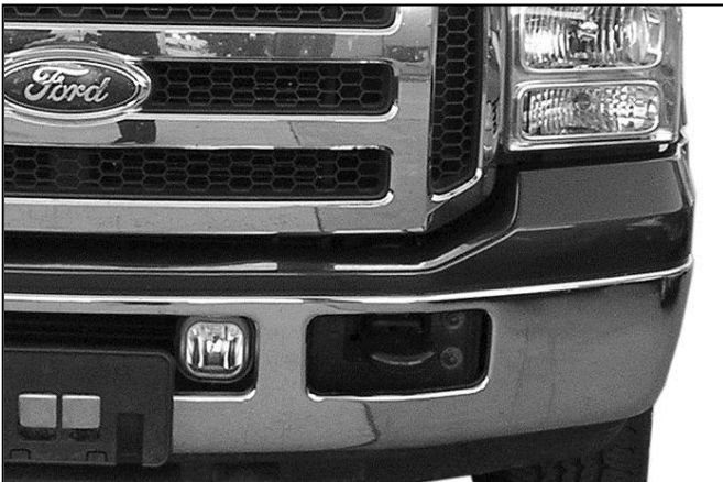
(Fig 1) unplug wire harness from fog light behind bumper
