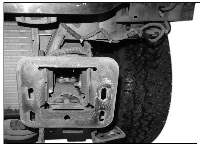
(Fig 9) Driver/left side frame mounting location
