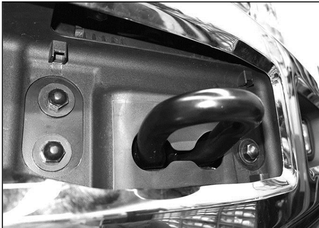
(Fig 6) Remove bumper bolts (driver side pictured)
