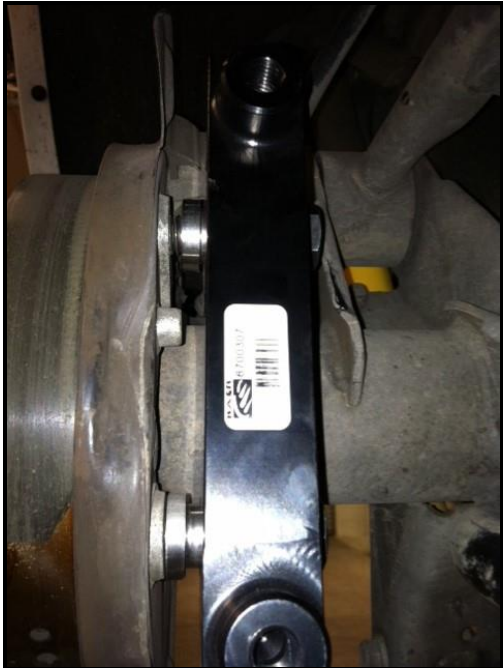
Bracket installed (slider heads mounted flush against flange)
