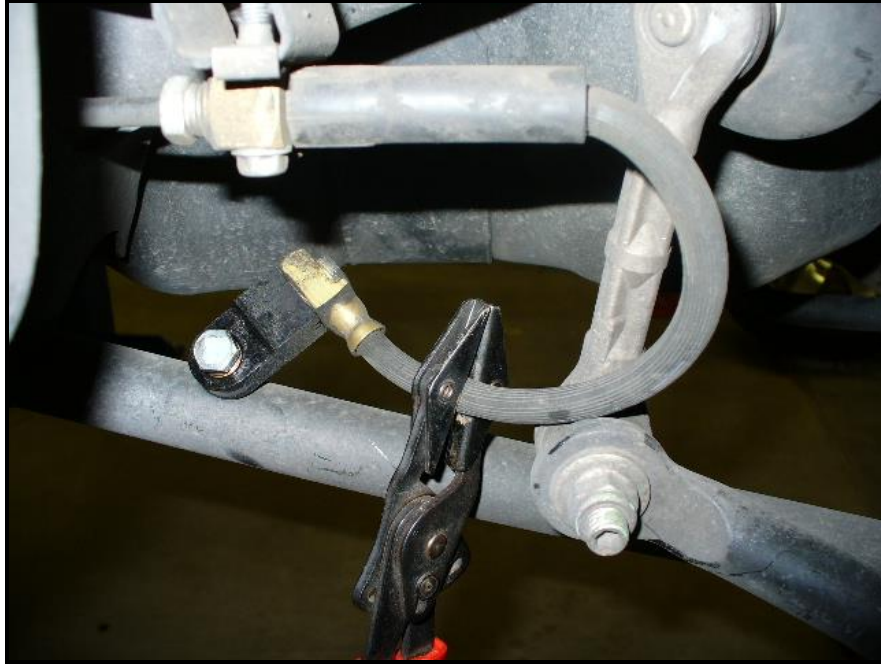
Line clamp to prevent brake fluid dripping during installation
