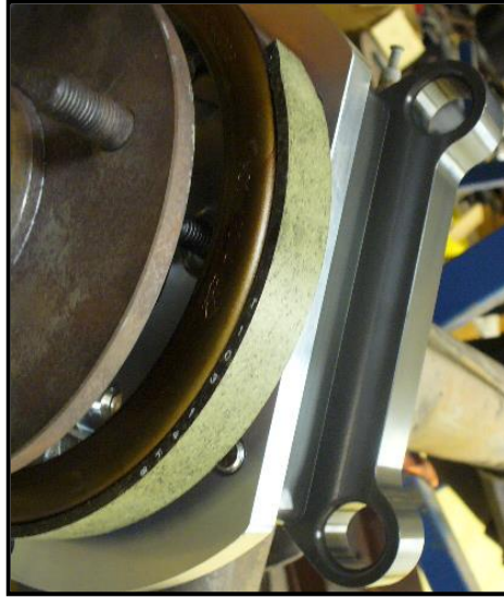
Park brake assembly correctly installed
