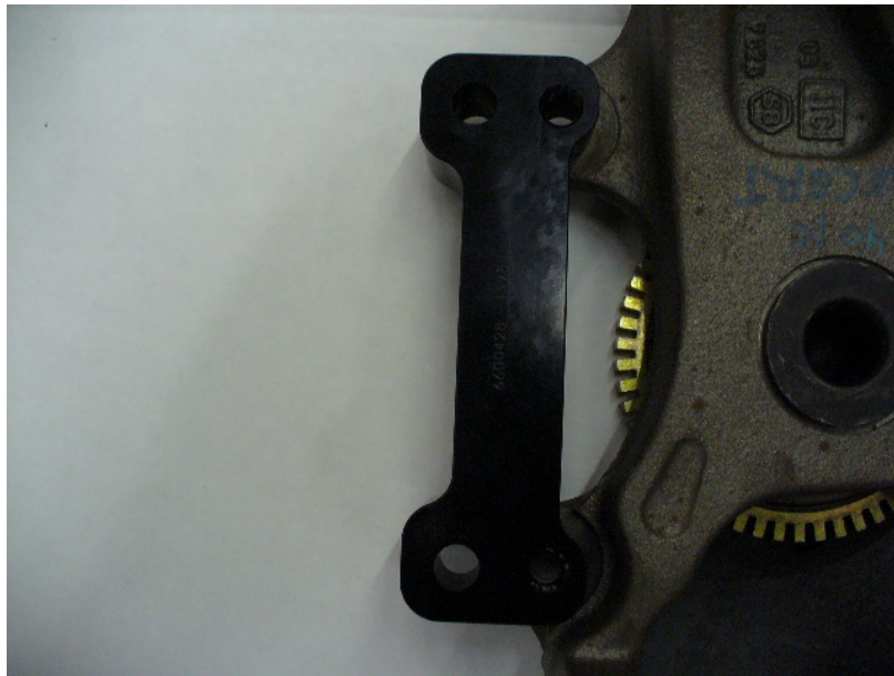
Bracket installed after caliper tabs trimmed.
