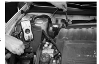
Positive Voltage Drop Test
