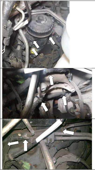
8. If you have a 2010-12 model year truck, you may have to remove the bolt holding the transmission lines in place to gain clearance for bracket access.
