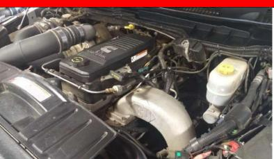
5 2. Place a pan or bucket below the fuel bowl and drain as much fuel out as possible by turning the drain valve. This will help reduce fuel spill when the fuel lines are disconnected. 3. Disconnect the fuel heater and WIF sensor connectors. 4. Disconnect the factory fuel quick connects from the fuel bowl, if still in use.(Fuel bowl shown removed for clarity) Note: Keep a rag handy, as more fuel may drain out of the bowl at this time.
