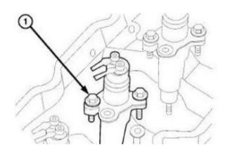
f. Do a final tightening of the fuel injector tube nut.
