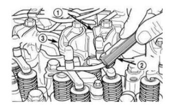
8. Reinstall rocker housing and cylinder head cover.
