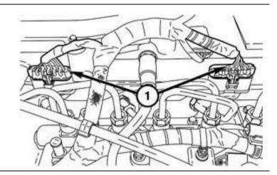
4.Remove all fuel injector wire harness nuts securing the integrated wiring harness to all fuel injectors.
