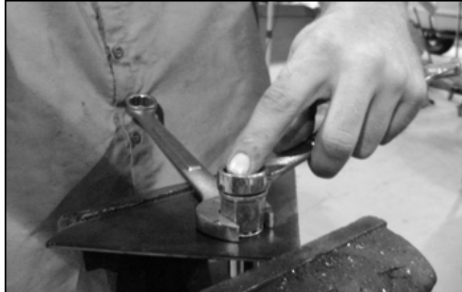
FIGURE 9 - 1/2" RIVET NUT SHOWN
