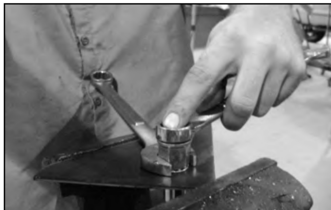
FIGURE 2 - 1/2" RIVET NUT SHOWN
