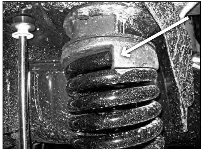
FIG 12B PASSENGER'S SIDE - INCORRECT
