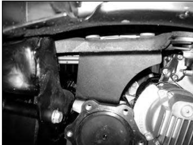
FIGURE 28 - SHOWN WITH DIFFERENTIAL ALREADY INSTALLED
