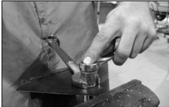
FIGURE 2 - 1/2" RIVET NUT SHOWN
