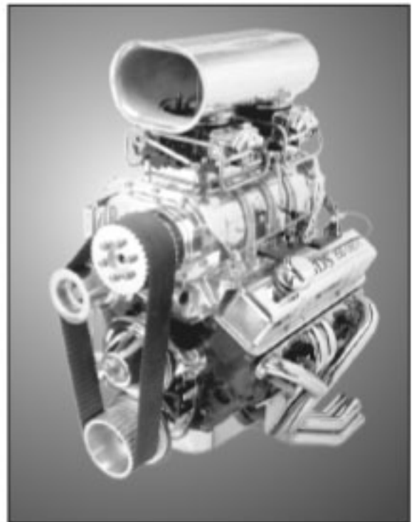
Chevy 350, 671, 1/2" pitch drive, dual carbs with scoop (right view)
