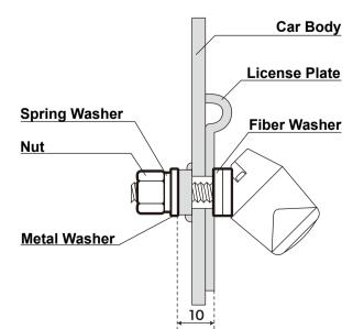
Thickness from the license plate of the vehicle to the back of the installation screw must be 10mm or less.
