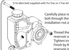
Carefully place reservoir onto pump, thread the 5/16" bolt through the reservoir and pump. Install the 5/16" installation nut and **finger tighten**.
