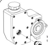
At this time remove the 5/16" installation nut and discard. Set the 5/16" allen bolt aside for
