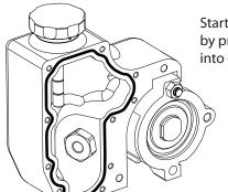
Starting at the top, install o-ring as shown by pressing o-ring straight down directly into groove.
