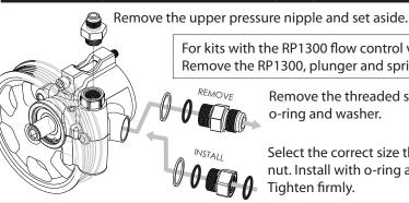
For kits with the RP1300 flow control valve installed. Remove the RP1300, plunger and spring. Set aside.
