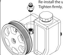
Re-install the upper pressure nipple at this time.
