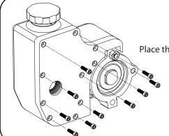
Place the reservoir back cover onto the reservoir.
