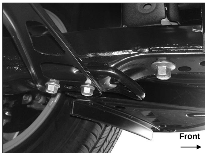
(Fig 6) Remove (2) 10mm hex bolts. Loosen but DO NOT REMOVE larger 12mm hex bolt. Pictured without splash guard for instruction purposes only
