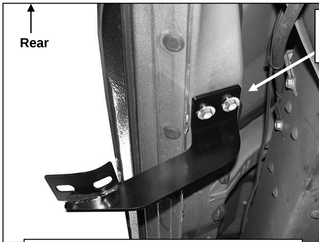
(Fig 5) Driver/Left Rear Bracket installed
