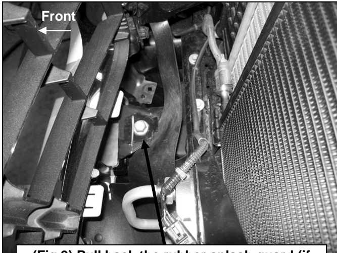
(Fig 9) Pull back the rubber splash guard (if equipped) to locate the factory hex bolt in the top of the frame (passenger side pictured)
