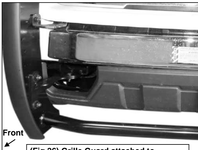
(Fig 26) Grille Guard attached to passenger side Brackets (pictured with MY 16-18 Top Bracket)
