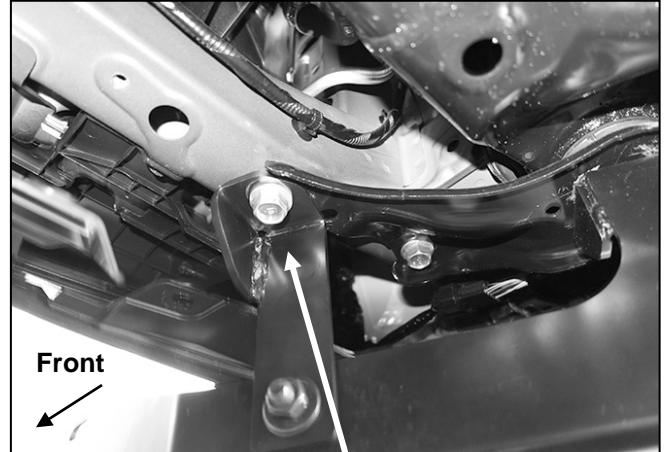
(Fig 4) Reuse factory hex bolt to attach passenger/right Support Bracket to cross member
