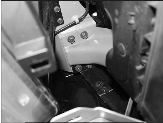
(Fig 11) Attach Top Support Bracket to top of Mounting Bracket
