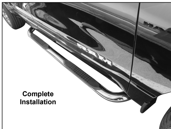
(Fig 12) Driver/left Front Brackets and Sidebar installed
