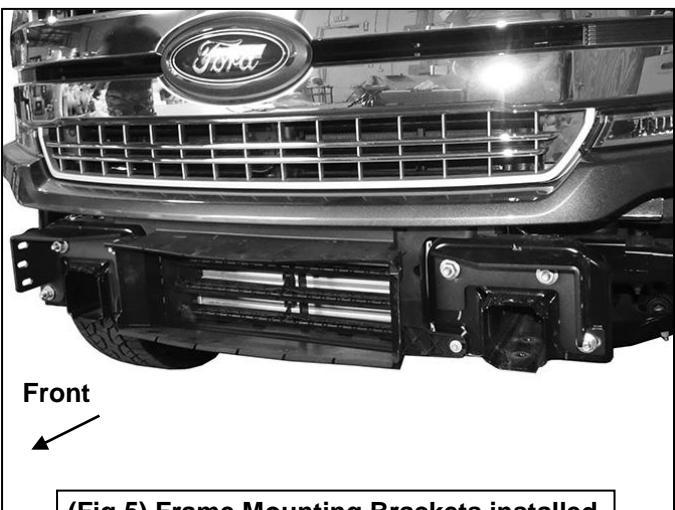
(Fig 5) Frame Mounting Brackets installed
